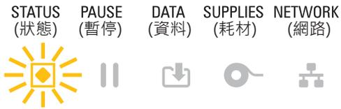
PRINTHEAD UNDER TEMP (印字頭溫度過低)
